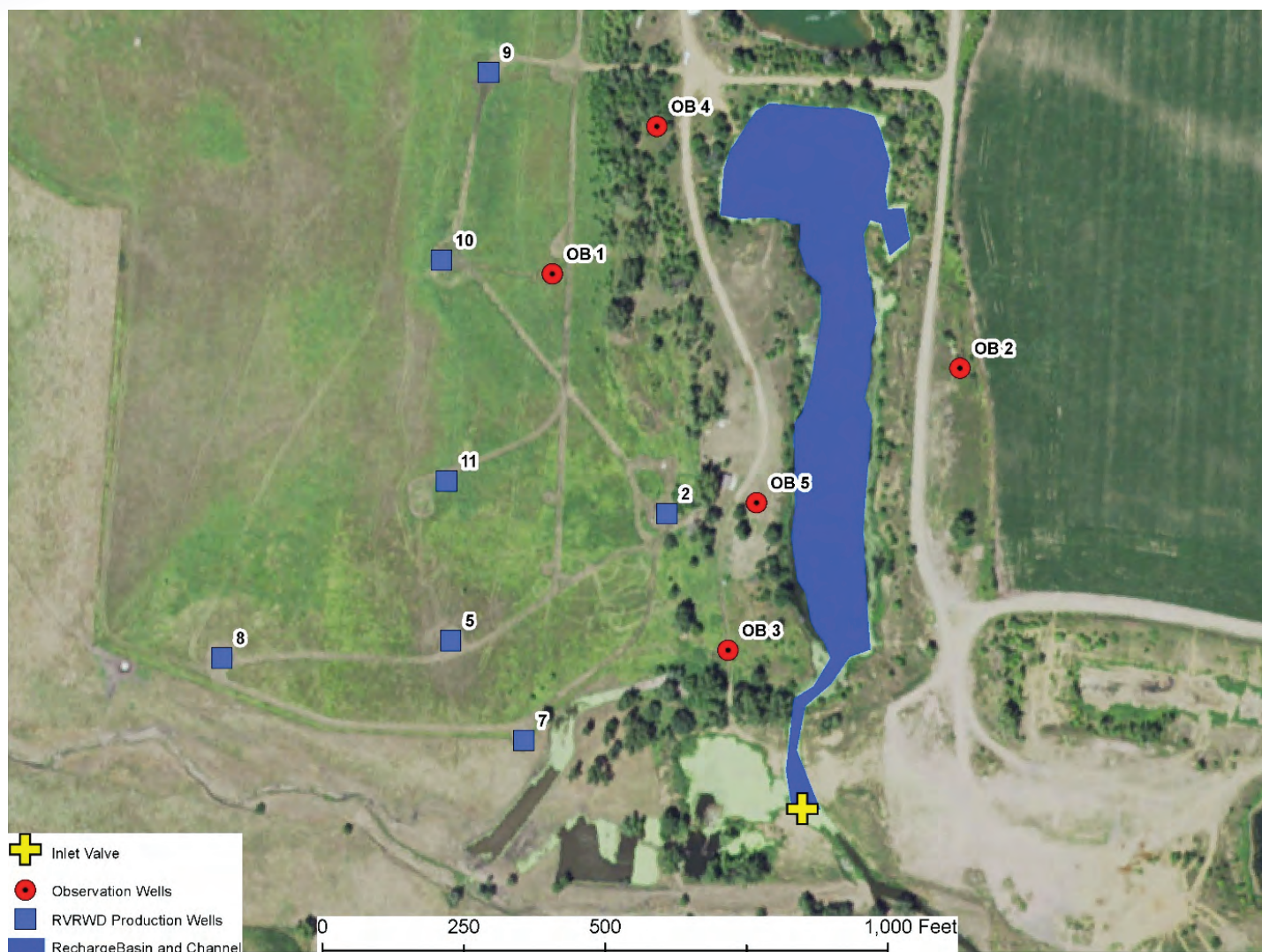
FIGURE 2: Sand and gravel quarry converted into a recharge basin with an unnamed creek re-routed into the basin to provide a water supply.
