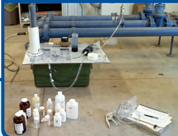
FIGURE 2. Typical sampling setup utilized for the groundwater study.
