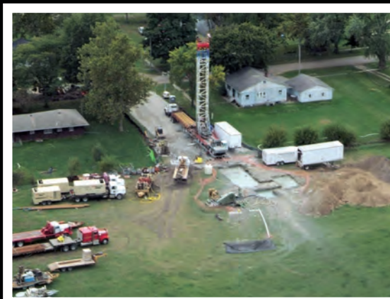
FIGURE 3. Drill site: Taylor 4000 HRT drilling rig – center; mud pit and Continental Emsco mud pump – left center; Ingersoll air compressors and booster compressors – left; various support vehicles for pipe, bentonite, tools, etc.
